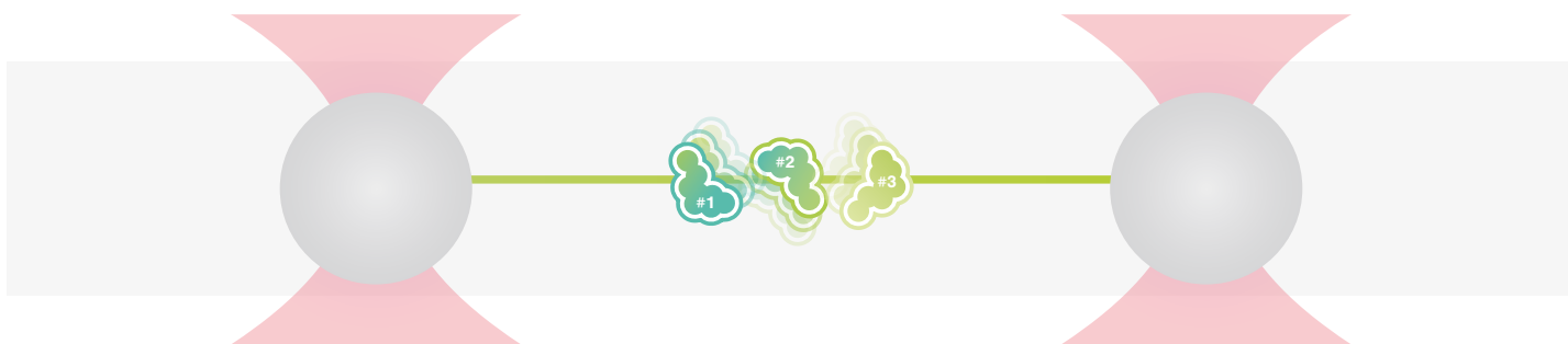
1 A schematic representation of a multi-domain protein unfolding experiment. A protein with three domains (#1, #2 and #3) is attached to optically trapped microspheres via DNA linkers.
